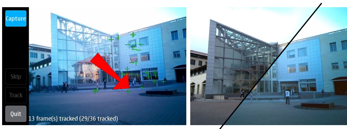
Figure 7.2: Rephotography. A Frankencamera platform makes it possible to experiment with novel capture interfaces directly on the camera. Left: The rephotography application directs the user towards the location from which a reference photograph was taken (by displaying a red arrow on the viewfinder). Right: The reference photograph (above and left), which was taken during the morning, overlaid on the image captured by the rephotography application several days later at dusk.
