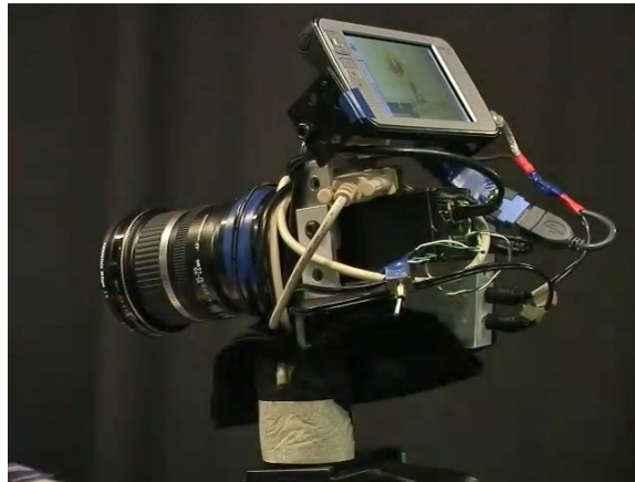
Figure 5.1: The F1 Frankencamera. The first experimental hardware platform, the F1 used an Elphel 10353 network camera connected to a Nokia N800 tablet. A Birger EF-232 lens controller allowed Canon EF and EF-S lenses to be used, and a custom power supply allowed for portable use.
