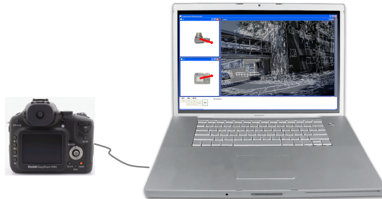
Figure 2.2: Rephotography with a tethered dSLR. In order to assist a photographer with the task of rephotography, where a historical scene is photographed again some time later from the exact same viewpoint, Bae et al. [38] were forced to run all computation and the user interface on a laptop connected to a dSLR, instead of on the camera itself. Figure courtesy of Soonmin Bae.
