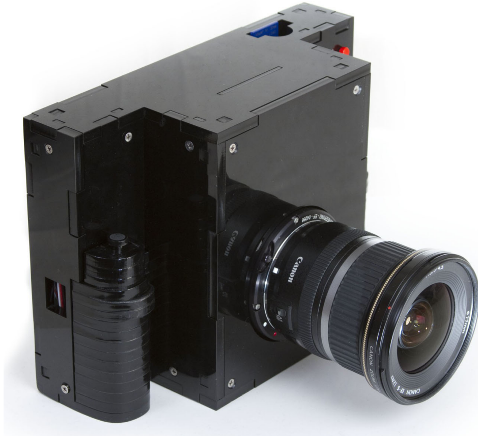
Figure 5.2: The F2 Frankencamera. A portable 5-megapixel computational camera that uses Canon lenses.
